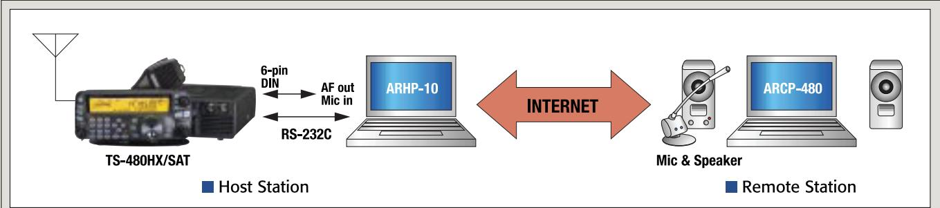
Using the ARHP-10 radio host program\*, you can even control the transceiver remotely over a LAN or via the Internet. The Kenwood Network Command System further enables VoIP (Voice over Internet Protocol) applications.
