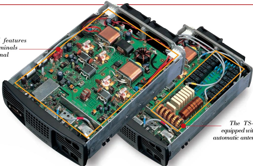
The TS-480SAT is equipped with a built-in automatic antenna tuner.
