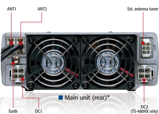
\*The TS-480SAT is equipped with a single fan.
