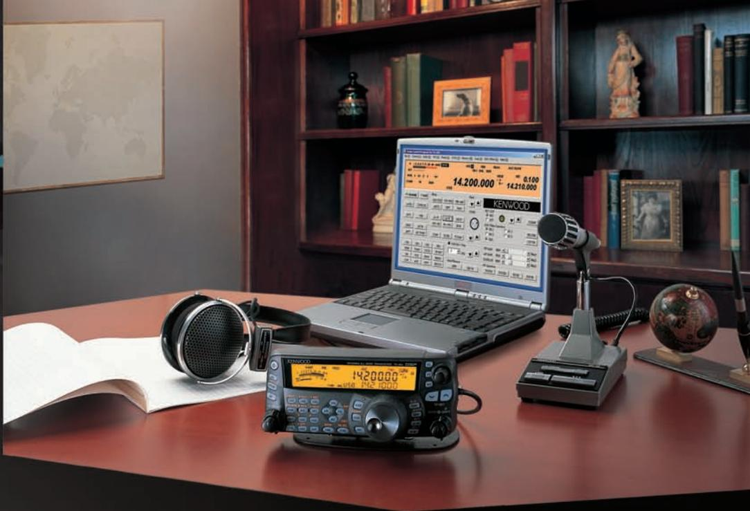
*Tailor-made for DX'ing, the new TS-480HX HF transceiver raises the bar on portable performance. Despite its compact dimensions, it delivers an astonishing punch: 200W with a DC 13.8V supply. Yet its separate control panel is perfect for base station use.*
