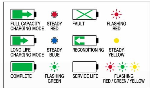
Battery conditions are displayed in colour illuminated indicators on the charger, which are also displayed on a connected PC with the same colour scheme. Colour-coordinated patterns provide users with at-a-glance information for comprehensive battery management.
